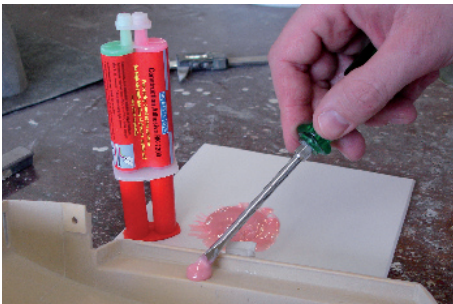
Bonding of plastic slats to shells made of glass fiber reinforced epoxy resin
