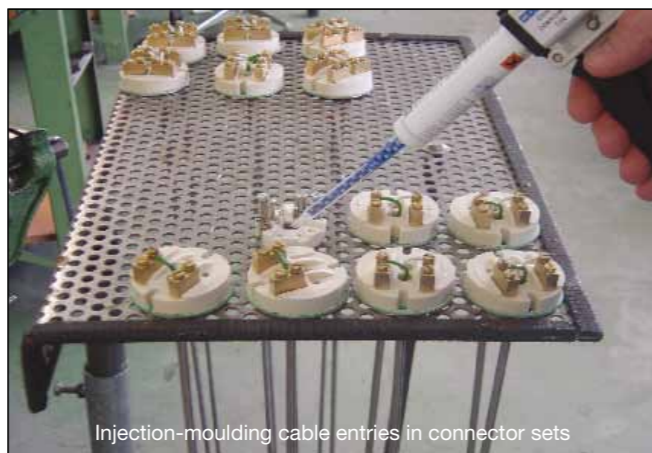
Injection-moulding cable entries in connector sets
