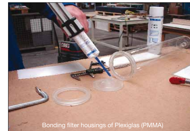
Bonding filter housings of Plexiglas (PMMA)
